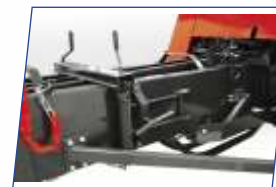
Four Way Bale Adjustment System
