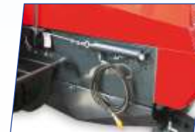
Hydraulically Adjustable Pick-Up Height Easy Operations
